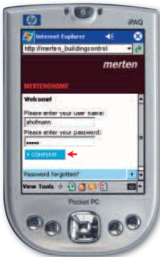
Step 1: Dial through to your home via the W-LAN hotspot using secure SSL-coded access.
